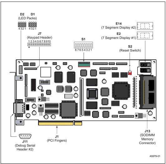
Figure A-2. S1, S2, LEDs, Keypad and Debug Headers and SODIMM Connector
