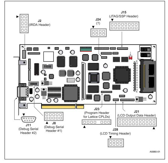
Figure 7-3. IrDA, JTAG, LCD, and Debug Ports and Headers
