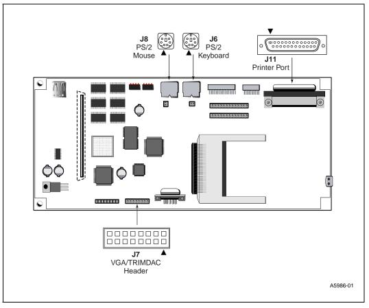
Header J7 is a combination of two connectors, an alternate VGA connection and TRIMDAC connections.
