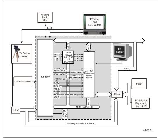
Figure 4-7. SA-1101 Development Board and SODIMM Board
