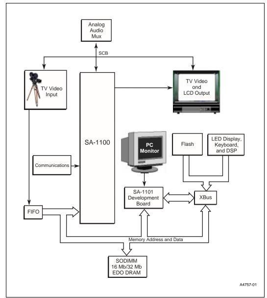
Figure 4-1. SA-1100 Multimedia Development Board Block Diagram
